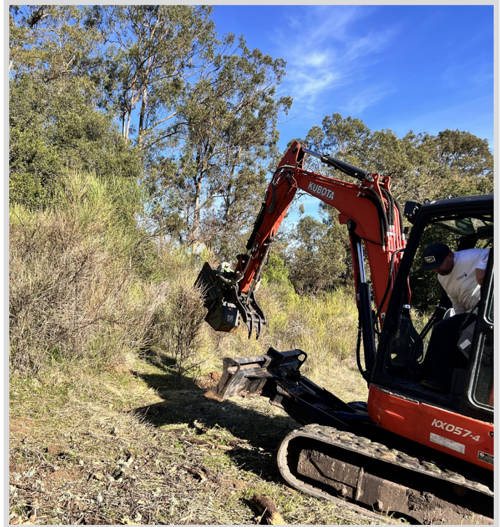
A fire brush masticator at work (heavy-duty mechanical tool designed to grind trees, brush, and woody vegetation into mulch)
